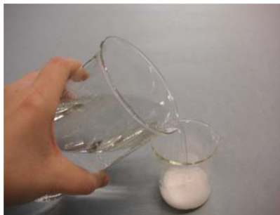
Add some of the mineral water to the Calcium Carbonate powder
