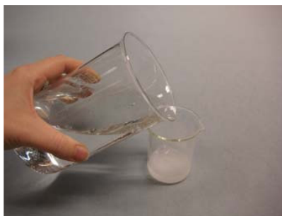
To clean, add some water from the 500 ml beaker into the 100 ml beaker, sway
