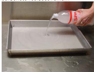
Pour the calcium bicarbonate into the treatment tray, keep some residue in the bottle
